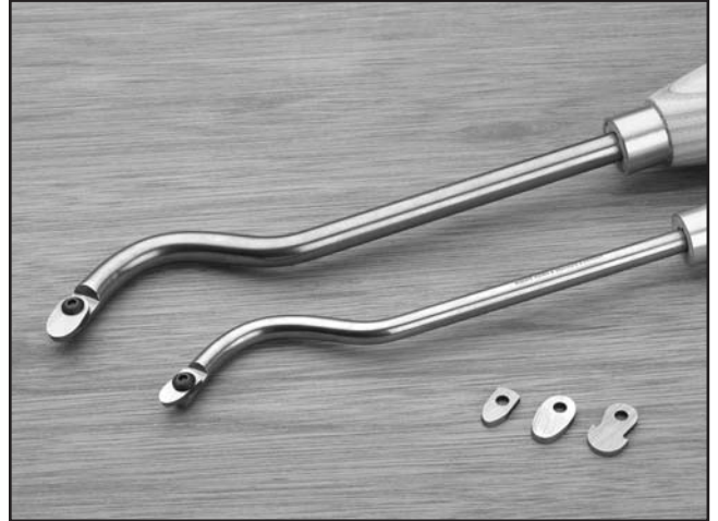
Figure 39. Swan Neck Hollowing Tools.
